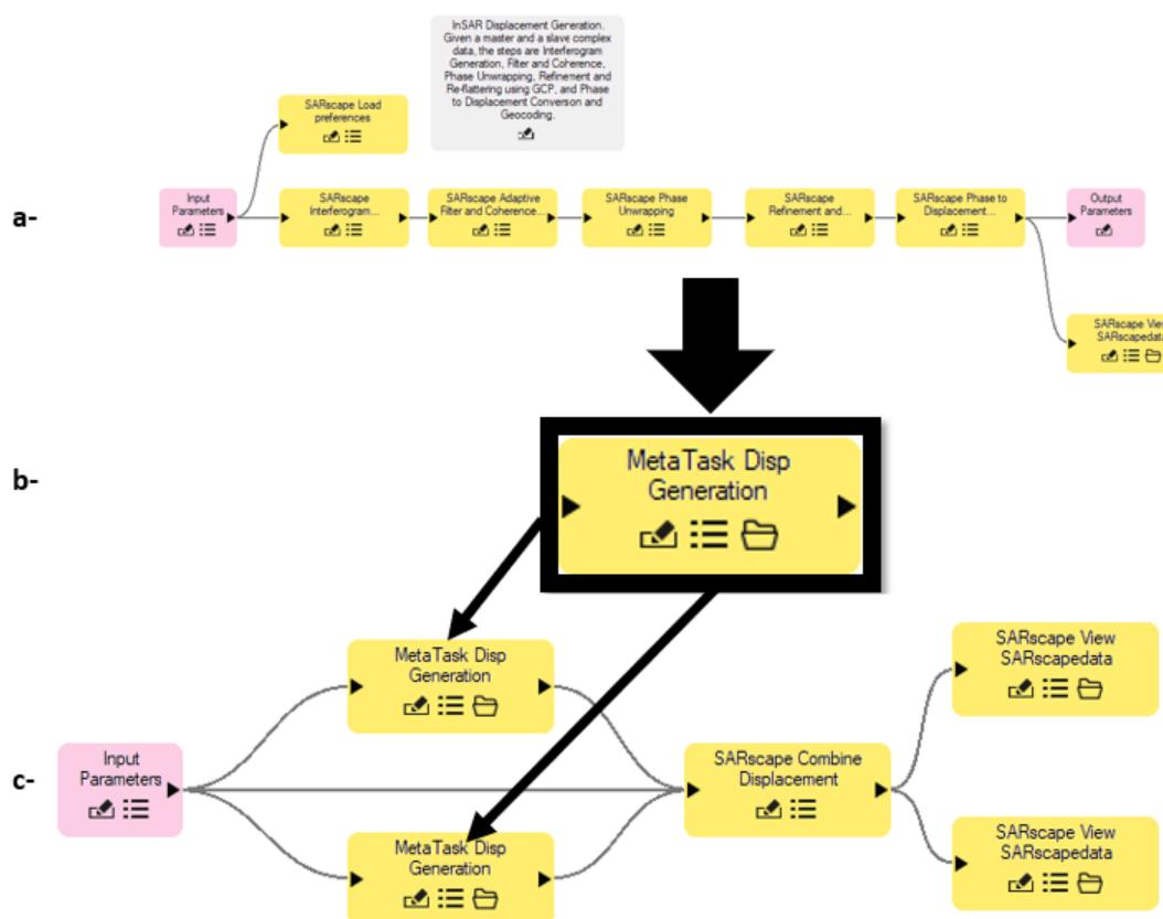
Figure 13 SARscape Metatask: a- Characteristic model look; b- Model collapsed in a Metatask. c- Metatask included in a new model.
