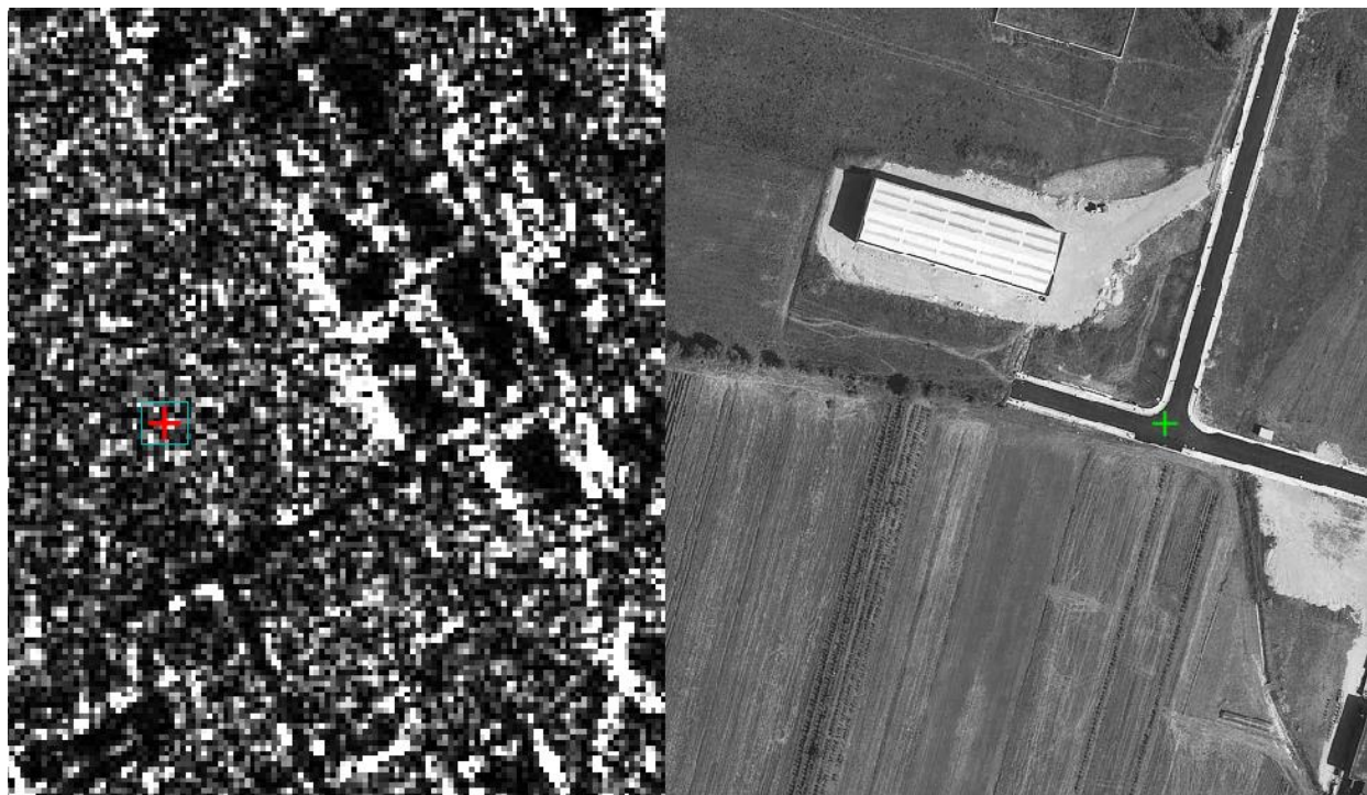
Figure 8: Center of the crossroad on the high resolution optical image (green "plus", right) and its wrong projection on slant range image (red "plus", left).
