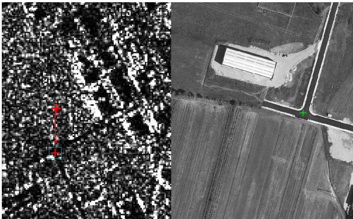
Figure 10: Change of position of the red "plus" on the slant range image (left) from the wrong to the correct position, in order to match the same location of the reference image (green "plus", right).
